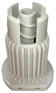
EnvisionTEC's ABS Hi-Impact Series is an extremely flexible ABS-like 3D printing material. It is an ideal solution for a wide variety of applications including snap-fit items and assembly applications which require some elasticity. It is a tough material, suitable for high-quality prototypes of items in categories such as automotive and consumer goods as well as stable enough for production-quaity end use parts.
