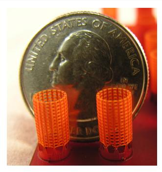
EnvisionTEC R11 is a liquid photopolymer that produces robust, accurate and functional parts. The material offers superior chemical resistance, a wide processing latitude, and excellent tolerance to a broad temperature and humidity range during and after build. Parts created from R11 exhibits superior fatigue properties, strong memory retention and high-quality up-facing and down-facing surfaces. For larger parts, please consider R5 as an alternative.
