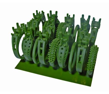
WIC100G resin was formulated for jewelry investment casting. The nano-wax content offers a clean burn-out with the highest reproduction of details. Wax casting is easy from WIC100G when using a standard wax burn-out cycle with a regular gypsum investment. During the burn-out cycle, the nano-wax melts away first allowing the resin to burn off without excessive expansion or pressure from degassing.
