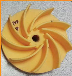
The pieces of the impeller are glued together for use as a pattern.
