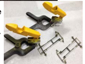
The halves of the body are put together, primed, and painted
