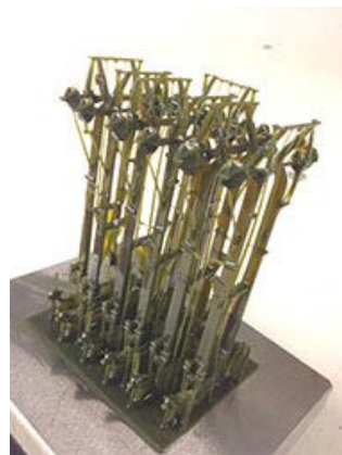
The chassis is arranged upright
