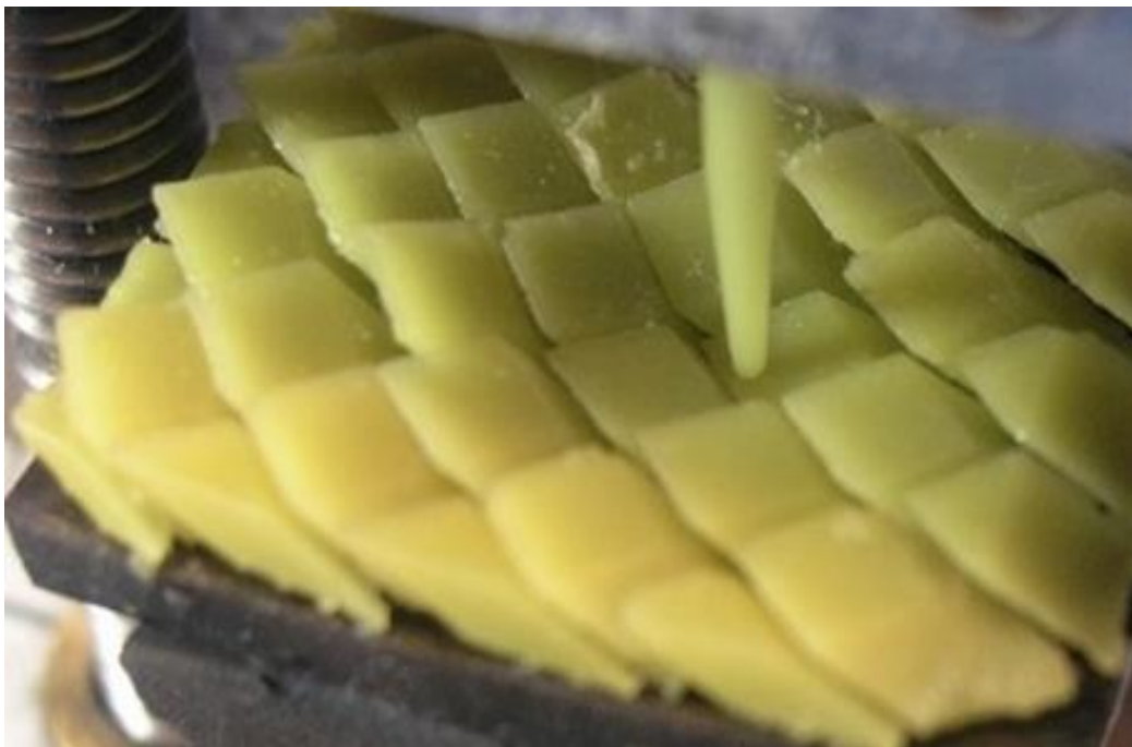
Elasmoid scales, 3D printed on the EnvisionTEC Micro Hi-Res, undergoing puncture testing. The EnvisionTEC printer enabled the McGill lab to determine the optimum scale designs for things like protective shielding on gloves.
