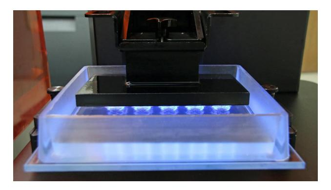
The new M-Type material tray for EnvisionTEC's Micro and Vida desktop 3D printers lasts about 3-4 months and is disposable. The bottom is optical glass coated in a film that allows for easy separation of exposure layers, surrounded by a soft but firm silicone frame.
