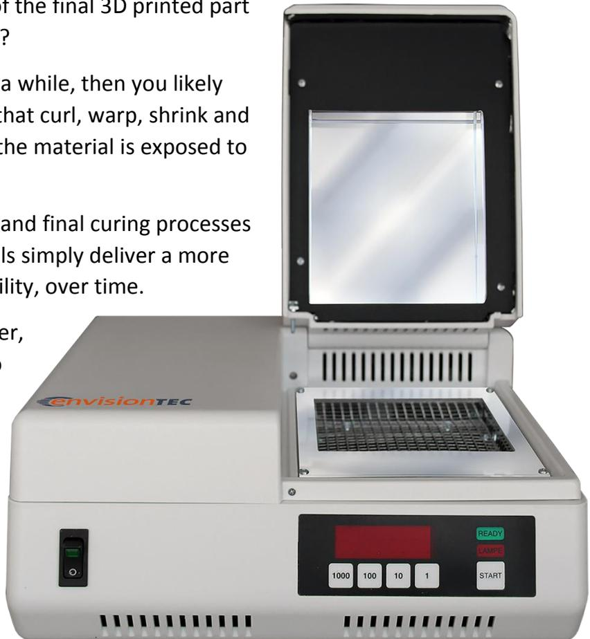
*To ensure that parts remain as stable as possible after 3D printing, EnvisionTEC provides specific post-curing instructions with its materials, along with specific post-curing technology, such as this OtoFlash. The lamps in this unit produce a very intensive light radiation in a spectrum from 300 to 700 nm. Because of this intensive light radiation, a better hardening of the materials is possible.*
