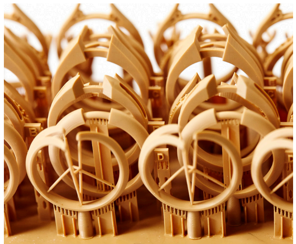
These ring patterns were printed on the Perfactory 4 in RC90. The resin allows them to build tough and stiff parts that are ideal for silicone molding.
