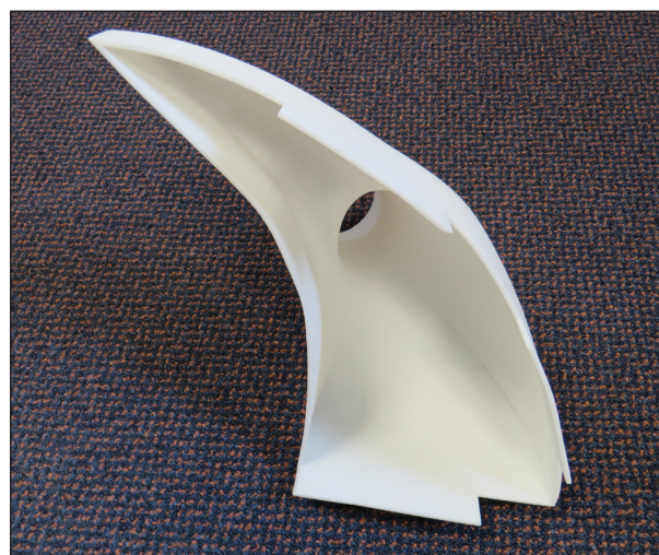
Team HARD GT4 Ginetta printed brake intake.
