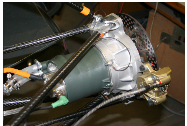
The water jackets produced by EnvisionTEC ensure that the motor stays cool and operating optimally.
