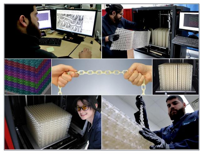
The EnvisionTEC Mega-Chain is a 328-foot chain that was 3D printed in a durable new material, E-RigidForm. Designed by EnvisionTEC 3D Builder Robert Montes (upper left and lower right), the chain features 6,144 links, each measuring 1.5 inches. The print job was processed with support from colleagues Erica Finkowski (lower left), Josue Nunes (upper right) and Jason Spurlock (not shown).
