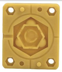
E-Tool 2.0 is filled with Barium Borosilicate Glass, known for its heat and chemical resistance, to deliver injection molds that can withstand high heat and pressure. Combined with EnvisionTEC's 3D printing technologies, E-Tool 2.0 delivers highly accurate tooling with an exceptionally smooth surface finish.
