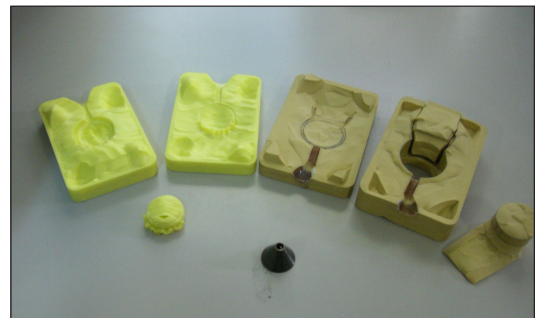
Prints can be produced for casting or the creation of silicone molds for mass production.
