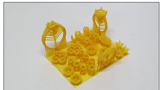
Multiple 3D prints are produced at the same time.
