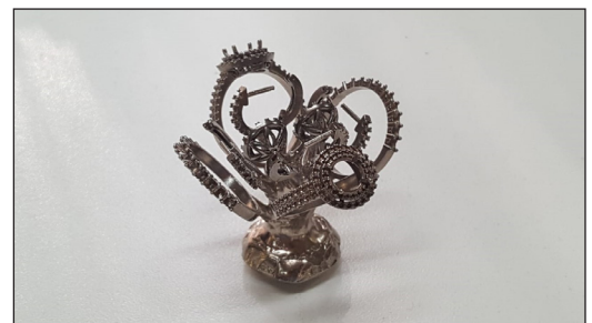
Once printed, objects produced in EnvisionTEC's castable materials can be easily attached to a sprue for direct casting.
