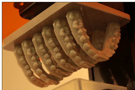
The large build platform size and depth allows the team to print multiple dental arches at the same time.
