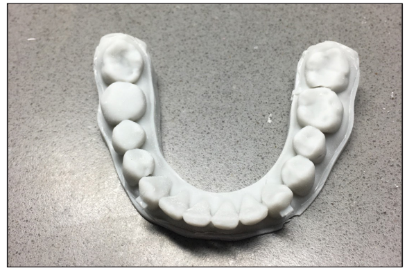
Highly accurate dental models are produced in a few hours on the Micro Plus XL.
