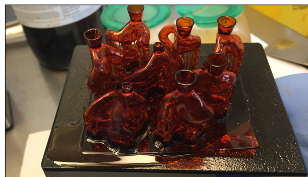
3D printed shells and molds are then printed.
