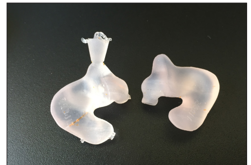
Soft silicone otoplastics molded from E-Silicone cocoon molds.
