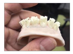
Printed veneers placed on a model. Still displaying the support structures from printing.
