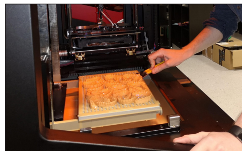
Dental models can be printed flat on the Vector 3SP and are easily removed (below).
