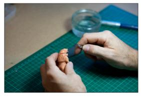
Any imperfections are easily removed prior the production of a mold.
