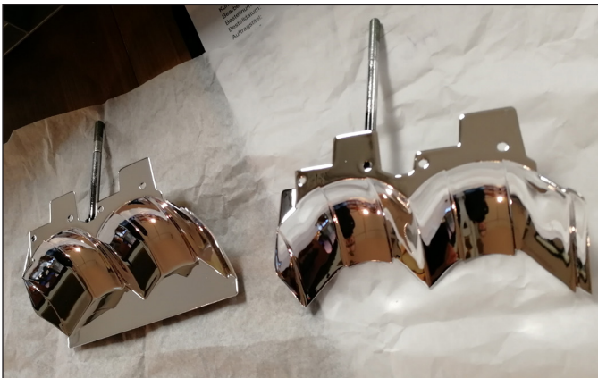
Light reflectors following plating.
