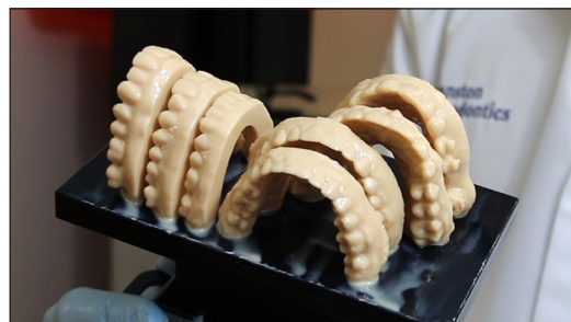
Below the printed arches are dried and cleaned.
