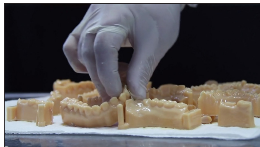
Below the printed arches are dried and cleaned.
