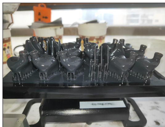
The large build platform on the Micro XL allows for the production of up to 7 ear shells in a single print. These can be printed vertically or horizontally to maximize yield.
