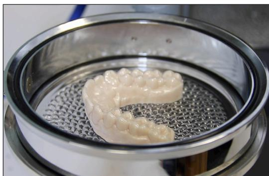
Once arches are printed, they are placed in the vacuum forming machine
