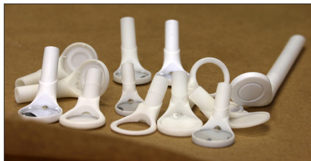
Multiple iterations of a prototype can be printed simultaneously. Speeding up the decision making process.
