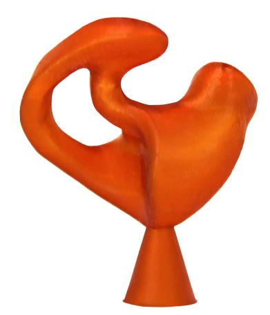
EnvisionTEC's E-Silicone material offers a solution to produce soft silicone otoplastics by the additive manufacture of cocoon molds. The custom fit E-Silicone molds may be injected with medical-grade silicone materials. The eggshell-like mold may then be easily broken away, leaving a soft, flexible shell. These shells can provide patients with increased comfort, better retention, better acoustic seal, more gain before feedback and improved sound quality.
