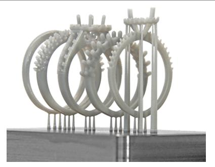
EnvisionTEC's quick building Q-View C resin is ideal for providing fast design verification models. This exciting material is capable of impressive print speeds on EnvisionTEC's cDLM (Continuous Digital Light Manufacturing) 3D printers.
