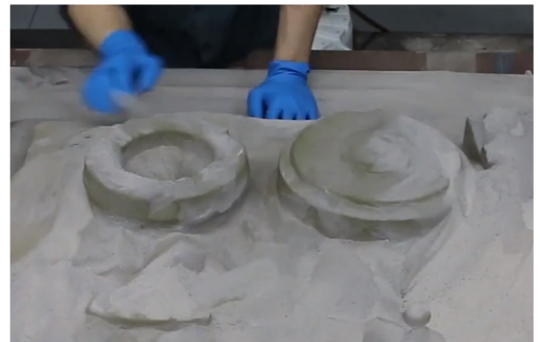
Finished cast items are quickly removed from the sand. Any left over sand is simply recycled for re-use in the Viridis.
