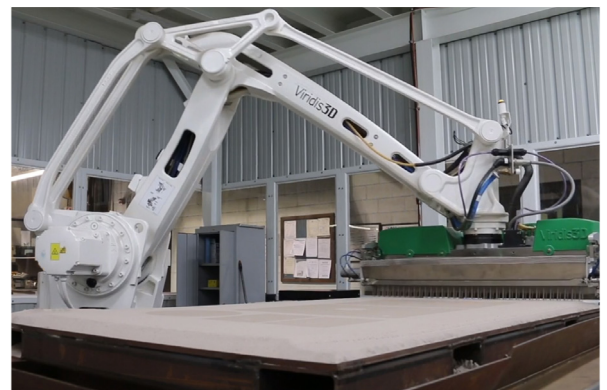
The Viridis RAM system printing.
