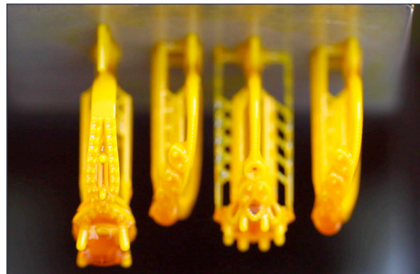
Extremely accurate models can be produced on the EnvisionTEC Micro cDLM in a matter of a few hours.
