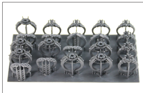
Large numbers of rings can be produced at once on the in house EnvisionTEC Perfactory series printer. Above, in EPIC castable material. Below, printed in Pro Gray which is ideal for creating master patterns for molding.
